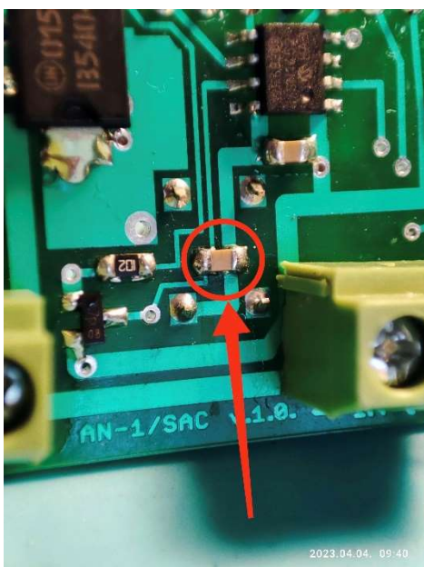
Picture #3 – capacitor is installed
