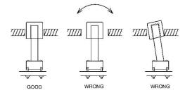
The correct size and position of pushbutton hole is important for flawless operation.
