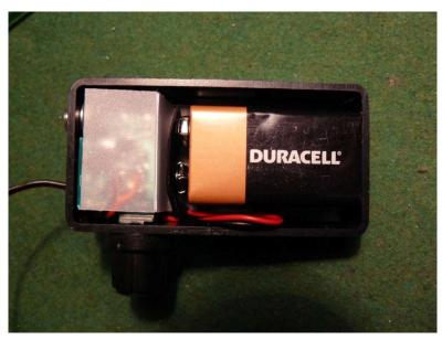
2. put the wire into the slot next to the battery, not on top of the battery
